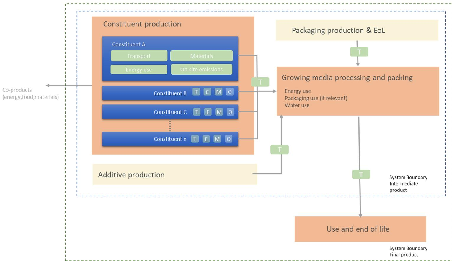
Figure 1 Simplified system boundary for a GMEFG study
